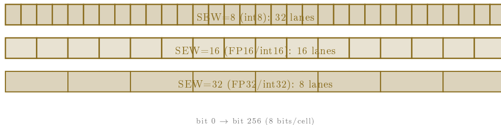
Figure 2: VSET 256-bit register lane layout — SEW selects the active row; all lanes operate in lockstep
